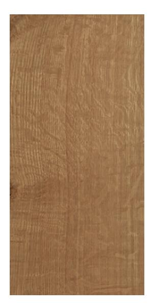
Quartersawn wood has a striking straight grain pattern that lends itself to design. Quartersawn lumber is defined as wood where the annular growth rings intersect the face of the board at a 60 to 90-degree angle. When cutting this lumber at the sawmill, each log is sawed at a radial angle into four quarters, which justifies the name. Dramatic flecking is also present in red oak and white oak.
